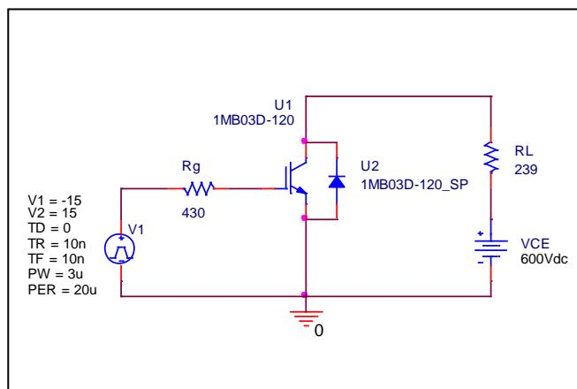
Test condition:  $I_C=2.5$  (A),  $V_{CC}=600$  (V)
