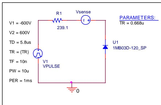
Test condition:  $V_{CC}=600$  (V),  $I_C=2.5$  (A),  $-di/dt=7.5$  (A/us)
